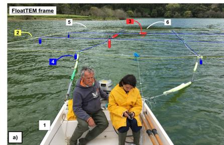
Fig. 3: (a) modified FloatTEM system with tube frame and boat. (b) underwater tripod (c) 3C-Uz-receiver.
