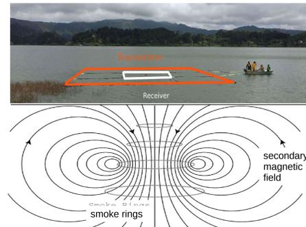
Fig. 2: FloatTEM system with tube frame and boat and the diffusion pattern of the signal in the subsurface
