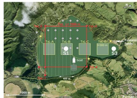
Fig. 4: Furnas lake survey design with transmitters (red, yellow) and receivers as gray dots and dashed lines
