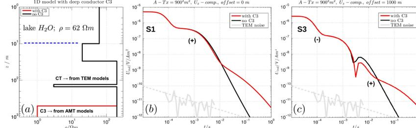
Fig. 5: (a) 1D model derived from AMT and FloatTEM results with and without C3 (b) secondary magnetic field in the center of the loop TxL (c) electric field at 1000 m offset for a dipole TxL-1
