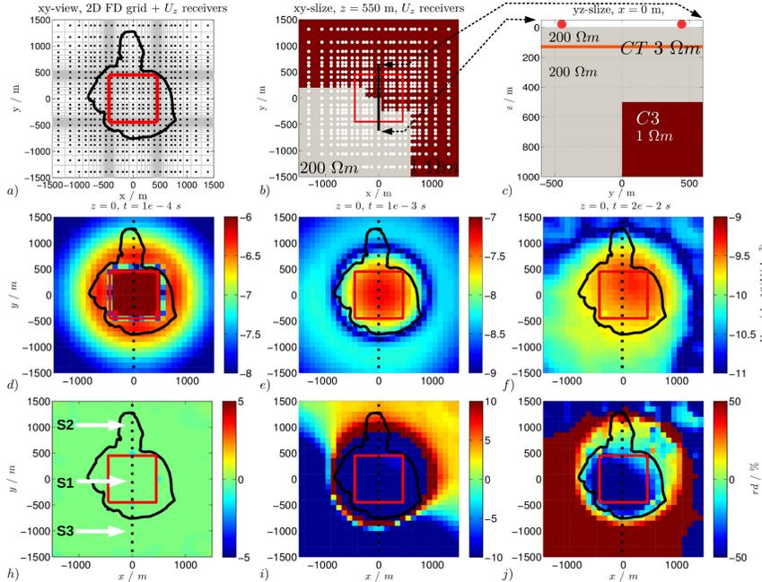
Fig. 6: (a) 3D survey setup for a large loop TxL and multiple receivers as dots (b,c) xy- and yz-slice with conductor C3 interrupted below the lake (d,e,f) xy- and yz-slice of the received secondary magnetic field for three transient times (h,i,j) relative difference of secondary magnetic field to response with a continuous C3.
