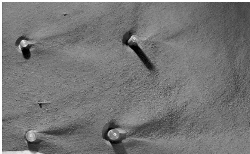
Fig. 6. Enhanced local wind erosion due to the presence of roughness elements observed in a wind tunnel experiment conducted by Shao in 1993 (unpublished).
